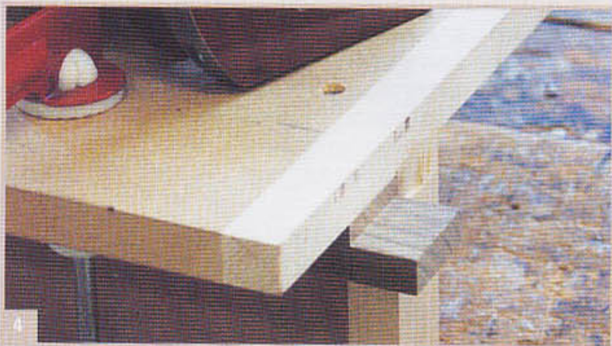
2 Tenoning jig set up
